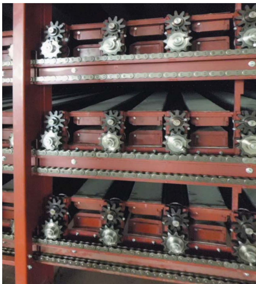
Interior of dryer (Roll driving side)
